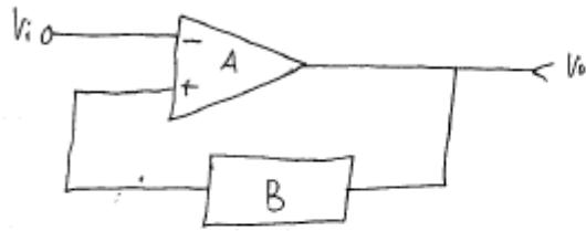
$$\rightarrow \text{positive feedback} : V_o = A(V_t - V_i) \quad ; \quad V_t = BV_o, \quad V = V_i$$
