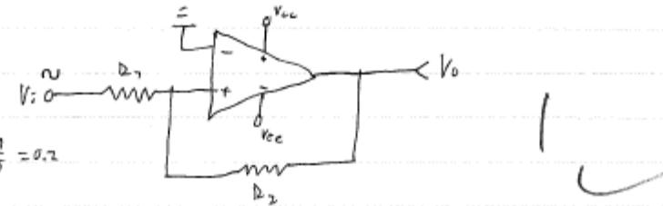
$$\frac{V_f - V_+}{R_1} = \frac{V_+ - V_0}{R_2} \rightarrow \frac{V_+ + V_0}{R_2} = \frac{V_i + V_0}{R_1}$$
