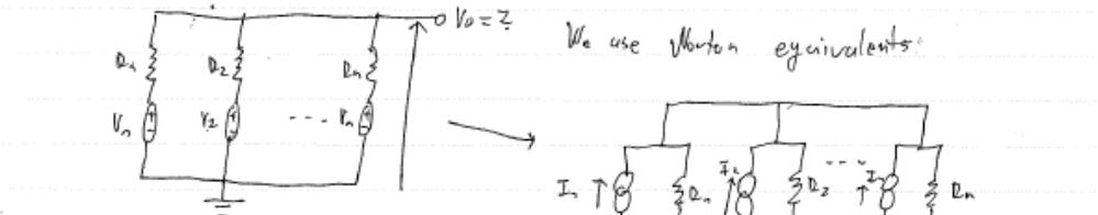
$$I_{\text{N}} = \frac{V_0}{R_n}$$
