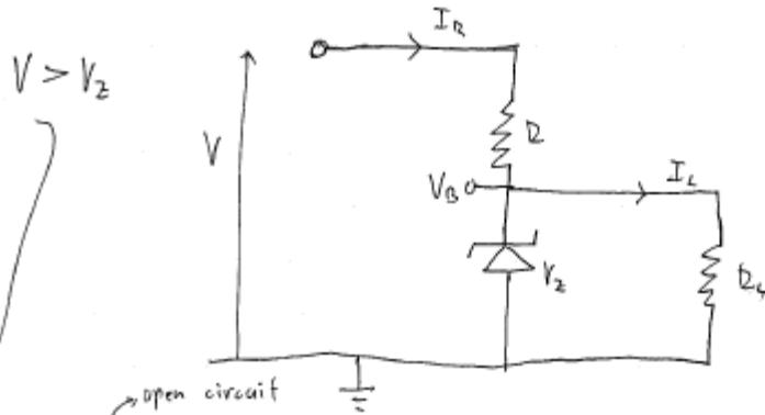
When Zener doesn't conduct:  $I_R = I_L$        $\frac{V - V_B}{R} = \frac{V_B - 0}{R_L}$
