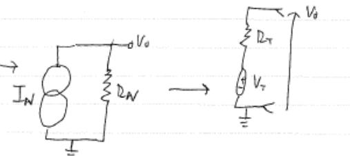
$$I_{\text{N}} = \sum_i I_i = \sum_i \frac{V_i}{R_i}$$
