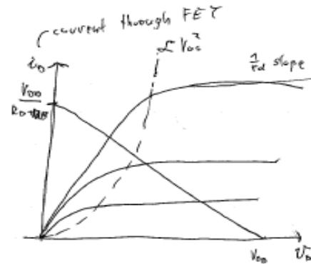
If  $V_{DS} > V_T$  then  $I_D = I_D(V_{DS})$
